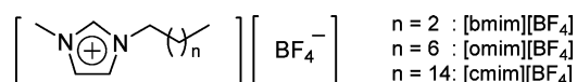
FIGURE 1. Imidazolium-based ionic liquids. bmim = 1- n -butyl-3-methylimidazolium cation; omim = 1- n -octyl-3-methylimidazolium cation; cmim = 1- n -cetyl-3-methylimidazolium cation.
